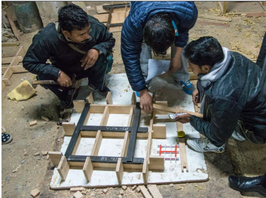
Calculating measurements for Jig C. Almost all of the jig parts were made with a hand saw and chisel. Note the white and orange 3D model of the jig. Photo: Ido Bruno
