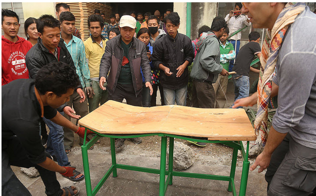
The Bhutanese manufactured Earthquake Desk withstood the 422kg crush test.
