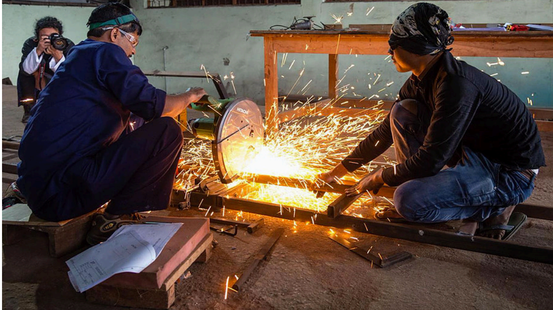
Cutting the first steel leg for the Earthquake Desk.
